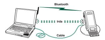
Local synchronization is done with either cable, infrared or Bluetooth wireless technology. The functionality is the same.
